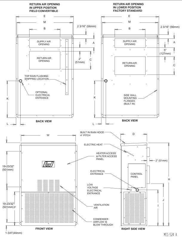
(\*) Position of return air flanges are interchangeable between two positions. Factory built at 5 inches (127mm).
